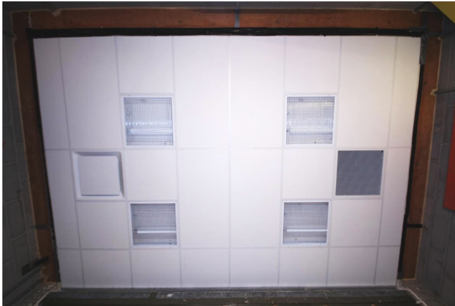
Typical ceiling system configuration used throughout the testing with various acoustic ceiling panels suspended in a metal grid and with light fixtures
